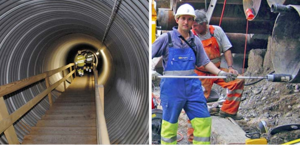
Transjura Motorway A16, construction of the section Roches-Moutier, Canton Berne. Trivec measurements in a pile wall
