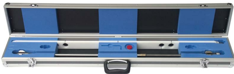
Sliding Deformometer in its case with probe guide
